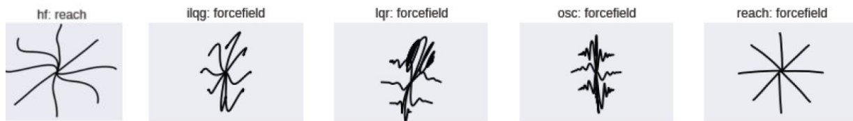
Figure 1: Force field reaching performance of several controllers compared. The REACH model performance (post adaptation) is shown on the far right. The deep learning (hf: hessian free) model (far left) generalizes poorly to other situations and training time proved to be too large for comparison of this controller on each of the tasks, we only show results for basic reaching. ilqg: iterative linear quadratic gaussian. lqr: linear quadratic regulator. osc: operational space control.
