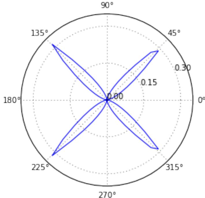
As we see the maxima of the error are aligned with the diagonals. By adding neurons with each diagonal as an encoder one after another the error gets reduced to zero:
