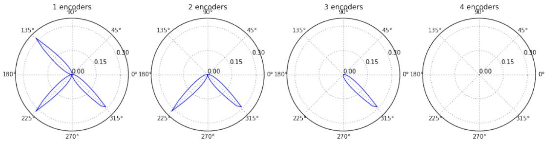
Using encoders with a different alignment will give worse results as the maximal possible reduction in error is less than for the diagonal directions. With those diagonal encoders instead of random encoders in the benchmark we obtain a substantial reduction of the error.
