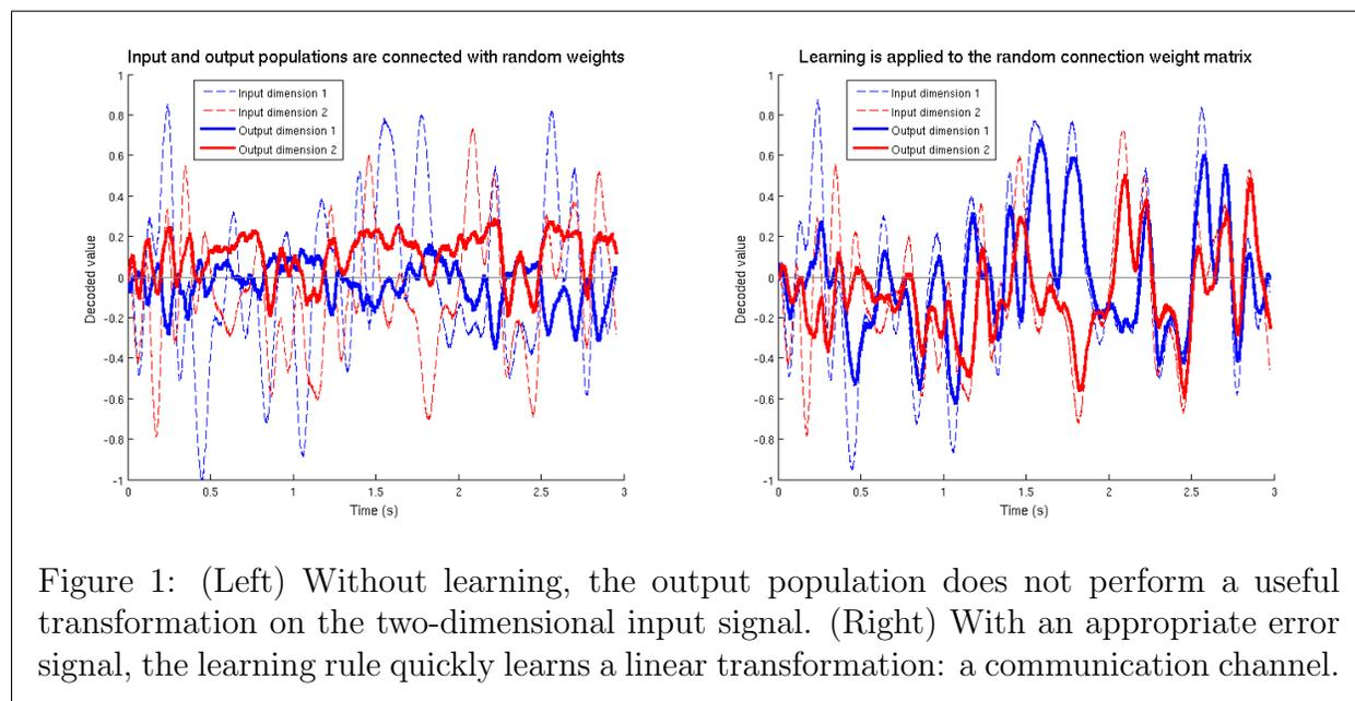
Figure 1: (Left) Without learning, the output population does not perform a useful transformation on the two-dimensional input signal. (Right) With an appropriate error signal, the learning rule quickly learns a linear transformation: a communication channel.
