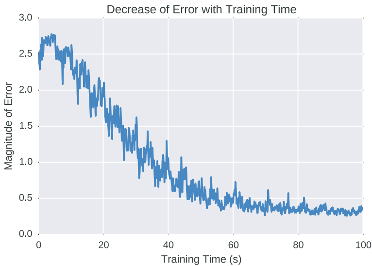
Fig. 5. Error magnitude in the Fast-Net decreasing with training received from the feedback of each trial.
